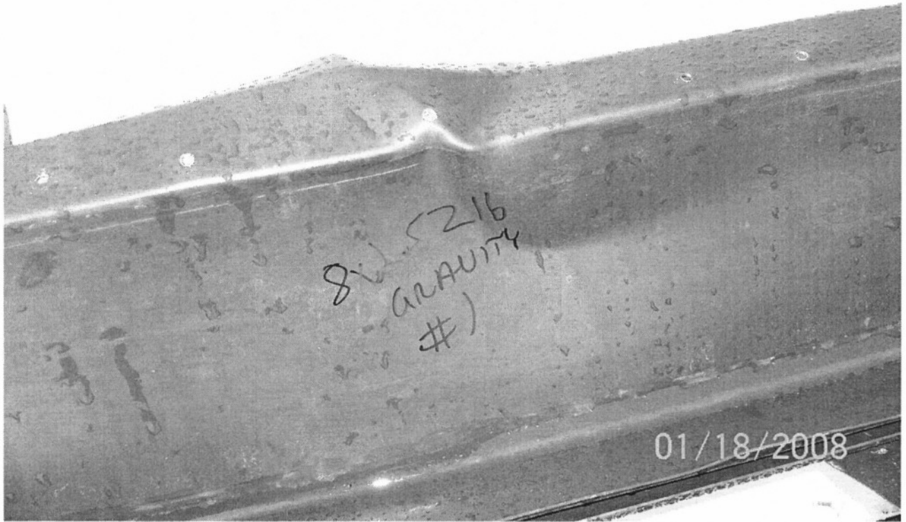
8X2.5ZEE 16 GA. TEST #1 FAILURE
