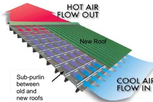
In the past few years, retrofit metal roofs have increased in popularity, which is largely due to recognition of their value based on tests conducted at the DOE's Oak Ridge National Laboratories. These retrofit systems, which create what is referred to as above sheathing ventilation (ASV), have proven to reduce the heat transmission through the new metal and existing roofs and into the building by as much as 45%. The ventilated
