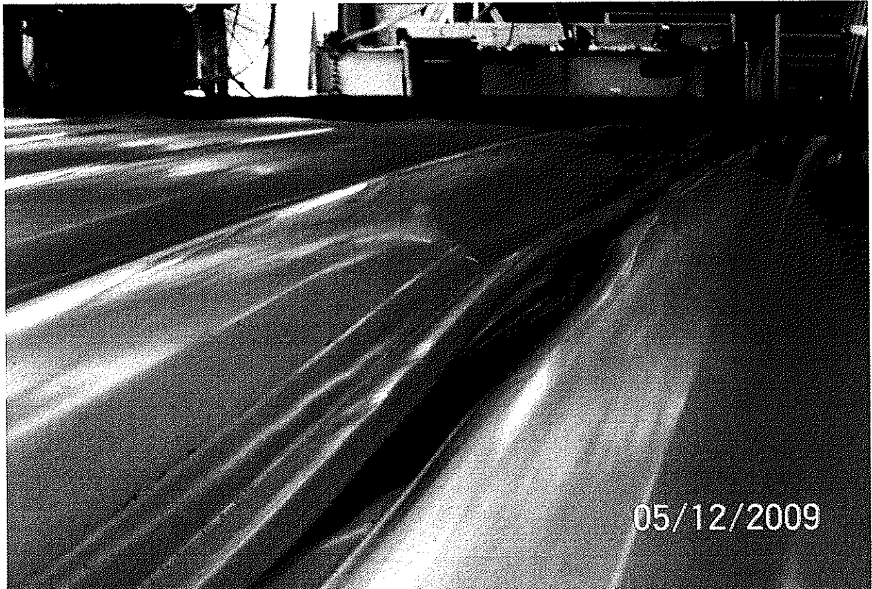
TEST C PANEL ASSEMBLY AFTER TESTING, SEAM DISENGAGED
