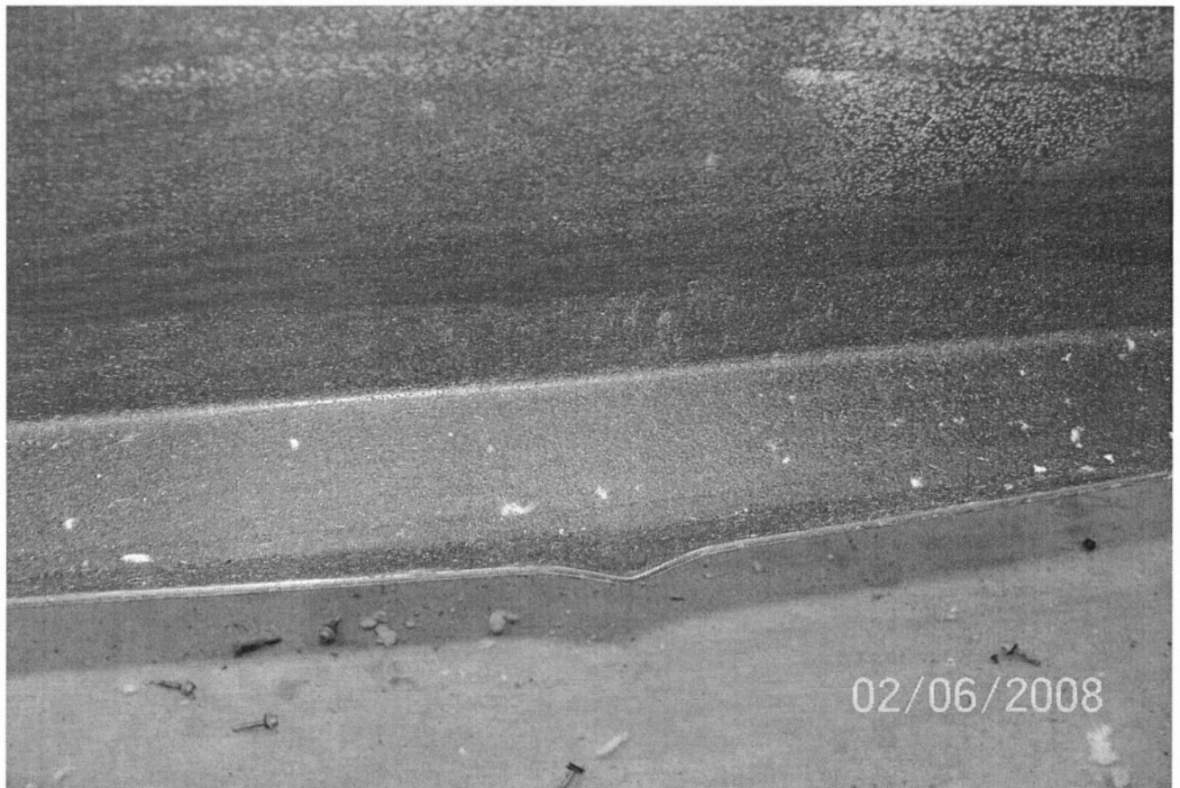
8X2.5ZEE 12 GA. TEST #1 FAILURE
