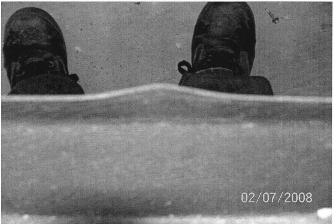
8X2.5ZEE 16 GA. TEST #2 FAILURE
