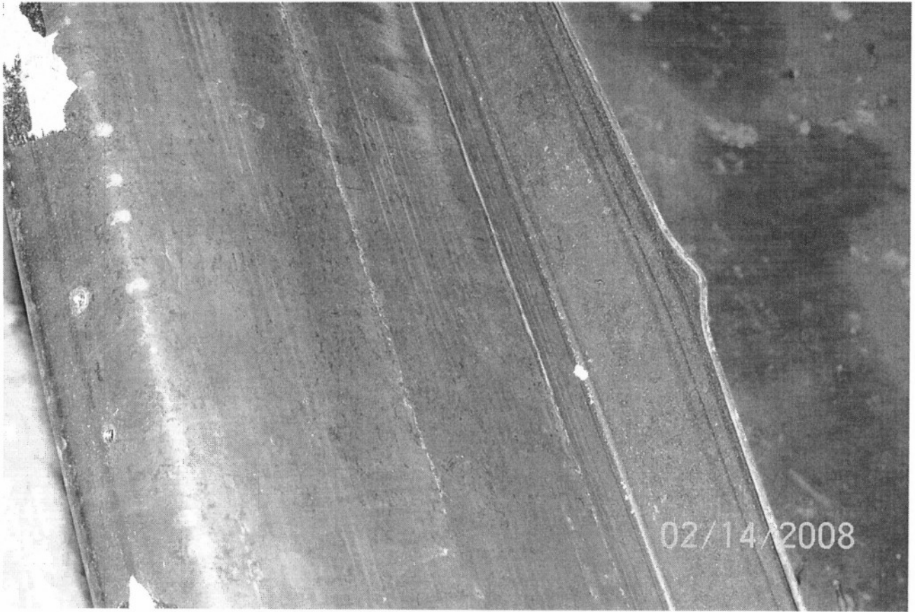
8X2.5ZEE 12 GA. TEST #2 FAILURE
