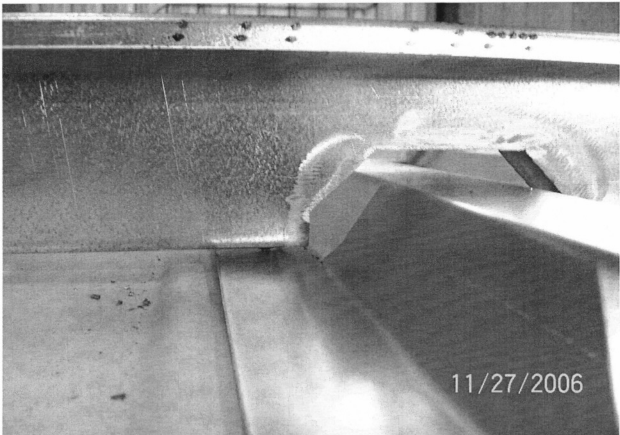
ASSEMBLY AFTER TESTING, TOPHAT PULLED OUT OF HAT SUPPORT
